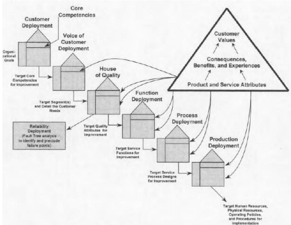
FIGURE 2. Adaptation of QFD for Extended Service Transactions.
