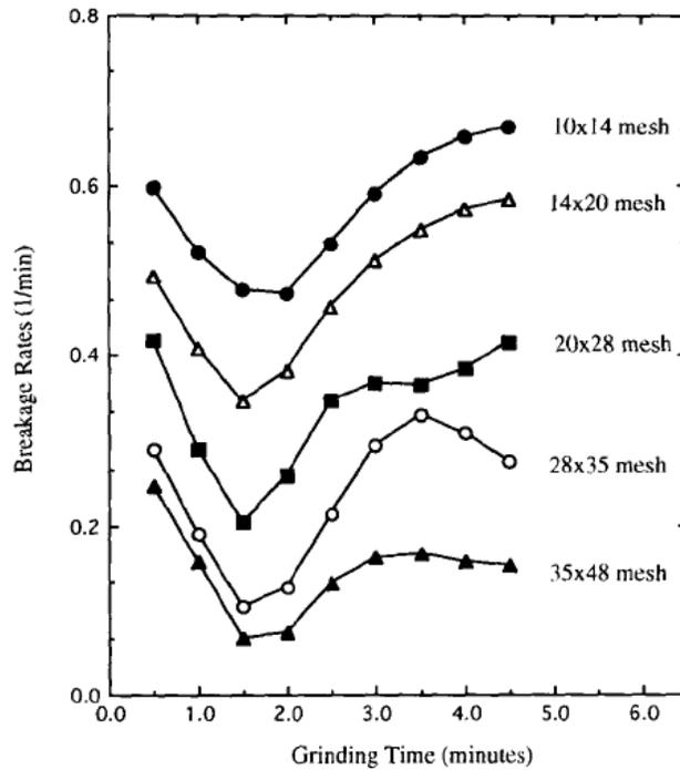
**Fig. 8.** Time dependence of breakage rates for a copper ore wet grinding experiment at 65% solids (natural size feed).
