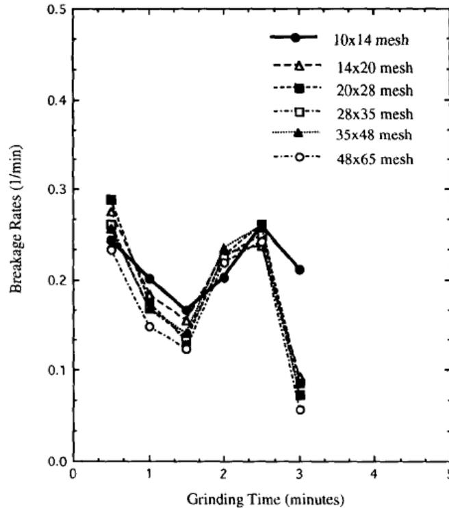
**Fig. 12.** Time dependence of breakage rates for a limestone wet grinding experiment at 85% solids (natural size feed); XFS4272 dosage: 0.03% on dry solids basis.
