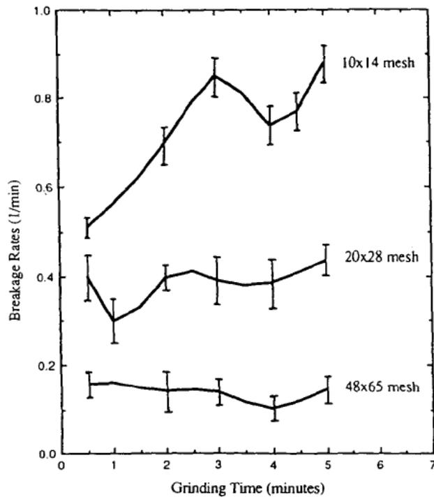
**Fig. 13.** Time dependence of breakage rates for a limestone dry grinding experiment. Vertical bars represent  $\pm 2$  standard deviation range (95% confidence interval) around the estimated breakage rates in the presence of 5% error.
