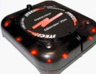
A handheld device (usually a "beeper" of some type) given to restaurant customers that alerts them when their table is ready. The device allows customers to move about a restaurant or a limited distance outside.
